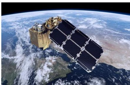
*Sentinel-2 satellite for wide-swath, high-resolution multispectral imaging*
